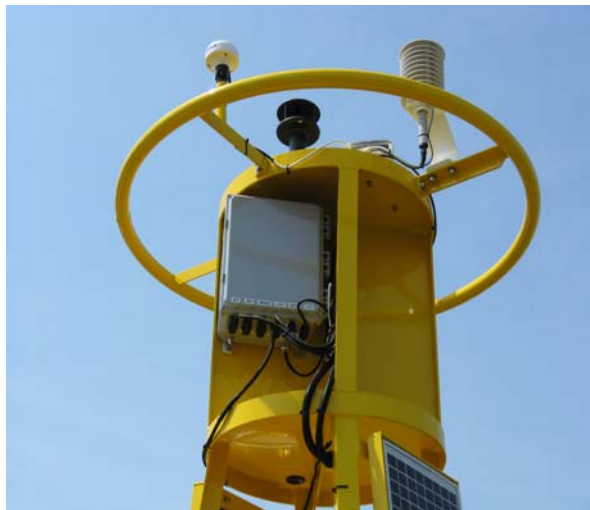
Tower section of a Down East MET Buoy showing sensors & watertight electronics enclosure.
